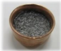
supplied in φ18mm Cu-cup form
