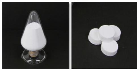
Appearance of the developed oxide-type solid electrolyte
